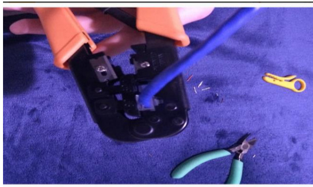
Fig 4.12: Crimp with RJ 45
