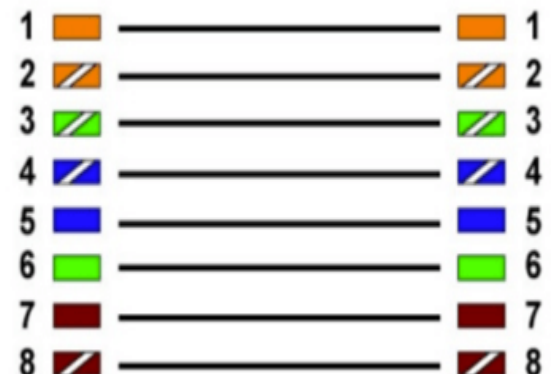
Fig 4.8: Straight through Cable
